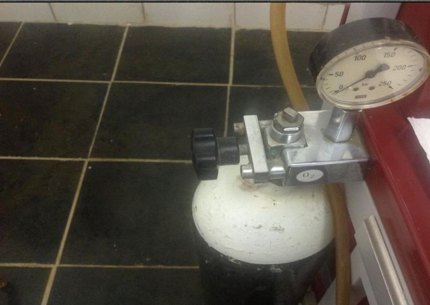
Dedza. Minor Theatre. Malawi machine. Empty oxygen cylinder, pin index.
